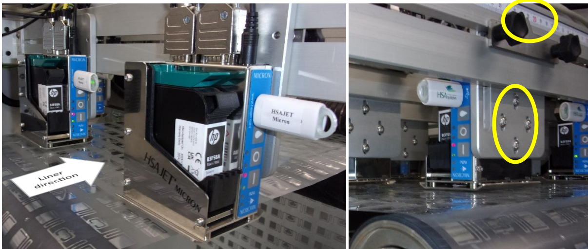
Figure 9. Example of bad tag markers with location indicators and height adjustment
