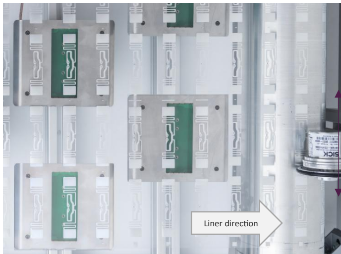
Figure 7. Snoop Pro mini coupling element mounted staggered under a multi-lane liner.
