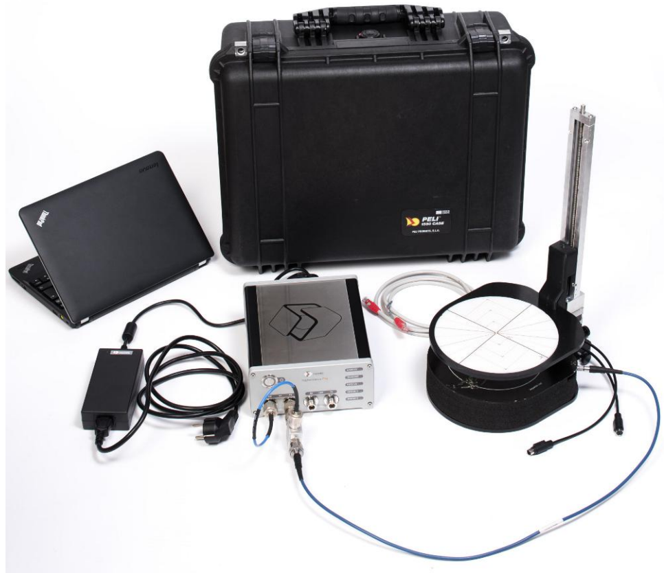
Figure 17. The basic Tagformance Pro and HCK HF measurement setup with the DCK
