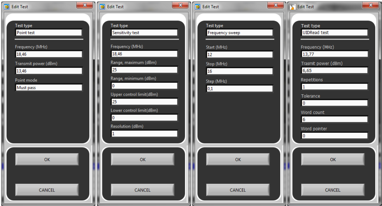
Figure 12: Add test dialog for Tagsurance HF target. When editing a test, the delete option will also appear
