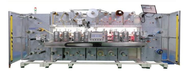
HOACO's RFID Label Converting Machine offers seamless handling of comlex RFID labels comprising more than four layers. The incorporated vacuum-based asynchronous inlay cut-n-transfer mechanism saves on process tapes and tooling costs. Additionally, the machine can be equipped
