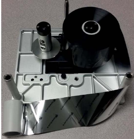
Figure 4-14: Ribbon Spools Removal
