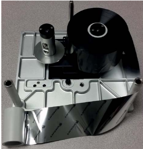
Figure 4-12: Ribbon Spool Installation
