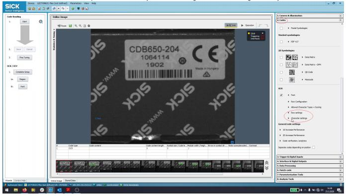
• Check optimal font size. Adjust camera distance if necessary to reach the best results. You may move the "Optimal font size" -caliper by clicking on the image window. The measuring tool is active in the "Edit image settings" window of OCR setup.
