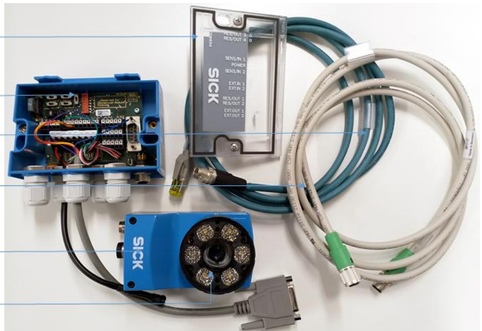
Fig 2. Sick camera and accessories added with extra D15 IO-connector and standard power supply connector with the integration box.
