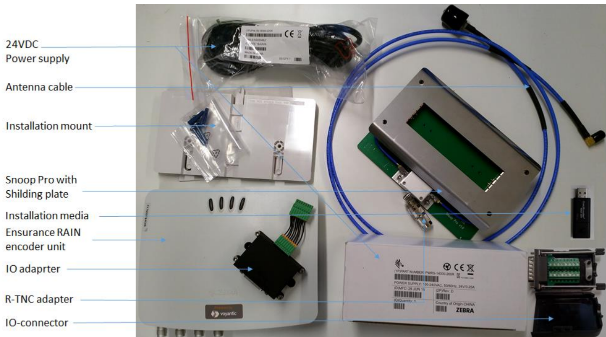
Fig 2. Ensurance RAIN encoder parts as provided with Realsurance Pro.
