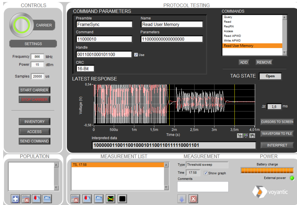
Figure 5. Attempting to read the user memory of a tag that does not implement the user memory. The tag responds to the Read command with a '1' bit meaning an error followed by an error code saying that the memory location does not exist.
