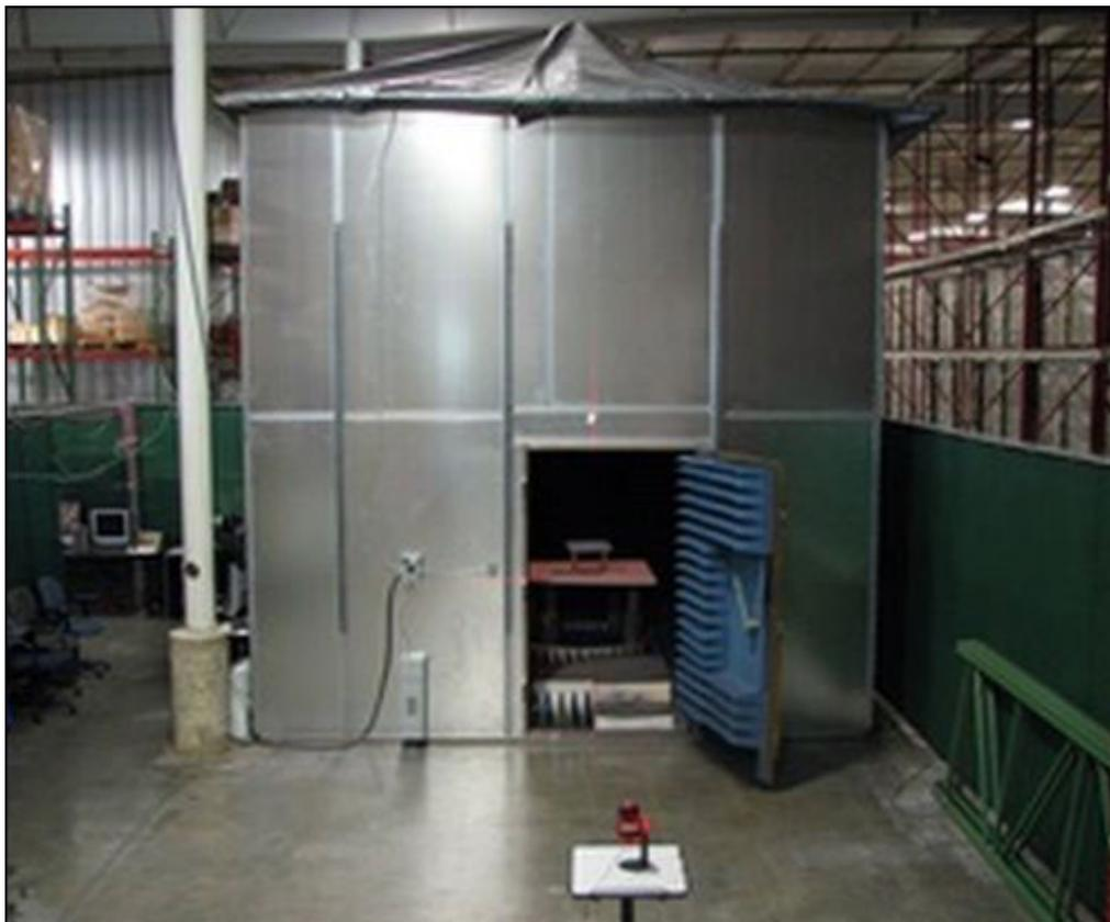
The ARC Center's testing chamber—a steel-clad structure measuring 12 feet on each side—has foam spikes that reduce the reflection of RF transmissions.
