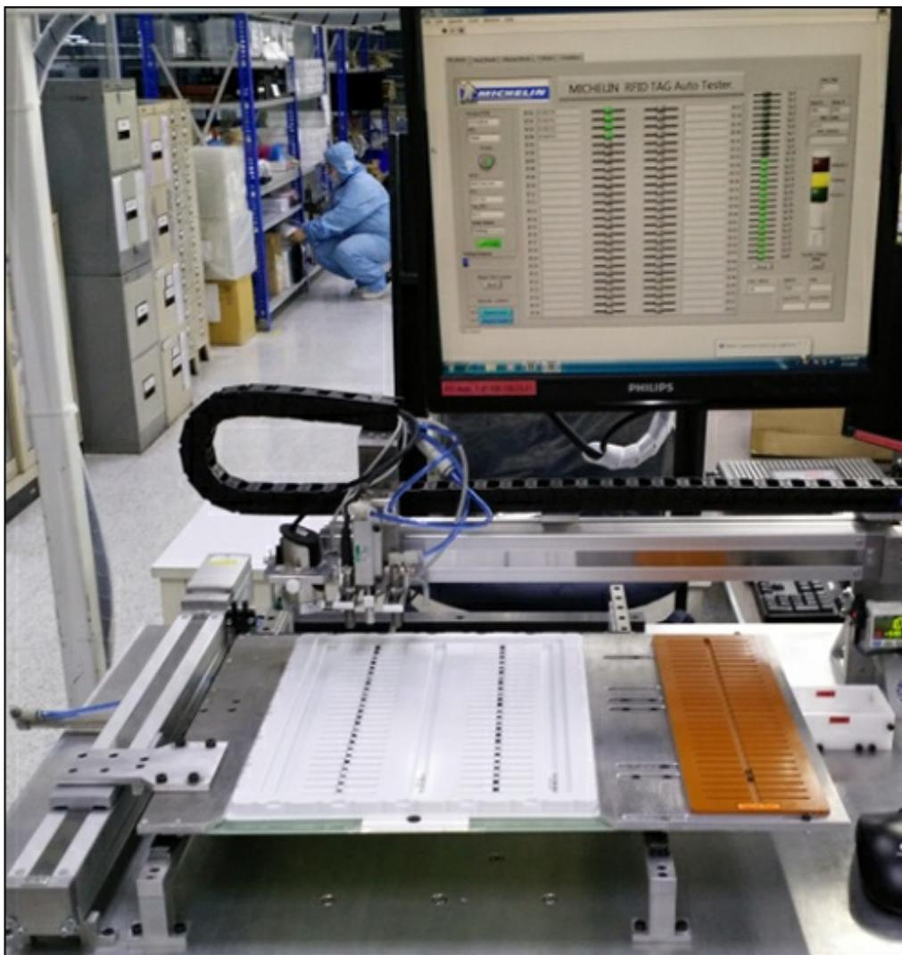
Before shipping the tags to the tire maker, Hana Microdisplay Technologies uses Voyantic's Tagsurance system to automatically test multiple tags loaded onto a tray.
